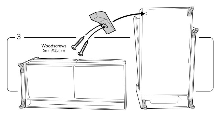
Attach each legs with the 2 (5mmX35mm) Woodscrews in the pre-drilled holes.
