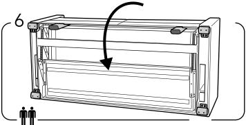
Mount the support leg in place and screw the 2 (M6X25mm) bolts into the pre-drilled holes.
