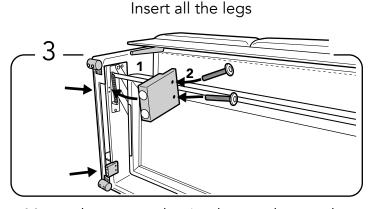
Mount the support leg in place and screw the 2 (M6X25mm) bolts into the pre-drilled holes.
