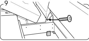
Attach the backrest to the chaise part (don't forget to use the two washers between).
