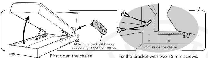
First open the chaise. Fix the bracket with two 15 mm screws.
