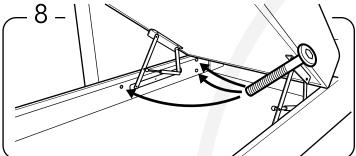
Fix the armrest with 3 bolts, one mount from frontside and two bolts mounts from backside.
