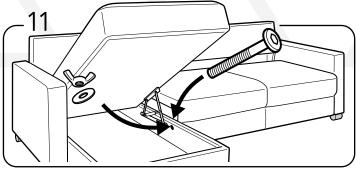
1st Close the bed mechanism. 2nd attach the bed at front with butterfly bolt set.
