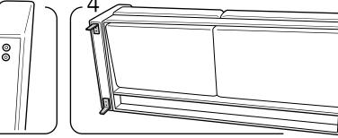
Mount the metal leg in place and screw the 2 (M6X25mm) bolts into the pre-drilled holes.
