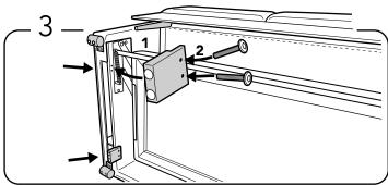
Mount the support leg in place and screw the 2 (M6X25mm) bolts into the pre-drilled holes.
