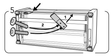
Mount the support leg in place and screw the 2 (M6X25mm) bolts into the pre-drilled holes.
