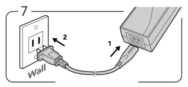
1- Connect the Wall Plug to the Power Supply.2- Plug the Power Supply Box in the wall.
