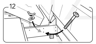
Mount the bed to openable chaise by using one bolt set on backside.
