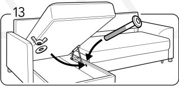
1st Close the bed mechanism. 2nd attach the bed at front with butterfly bolt set.
