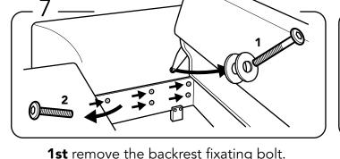
**1st** remove the backrest fixating bolt. **2nd** remove the 5 armrest fixating bolts.
