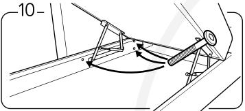
Fix the armrest with 3 bolts, one mount from frontside and two bolts mounts from backside.
