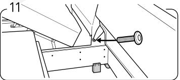
Attach the backrest to the chaise part (don't forget to use the two washers between).
