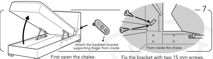
Fix the bracket with two 15 mm screws.
