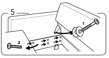
**1st** remove the backrest fixating bolt. 2nd remove the 5 armrest fixating bolts.
