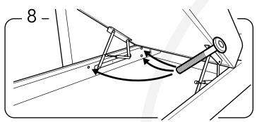
Fix the armrest with 3 bolts, one mount from frontside and two bolts mounts from backside.
