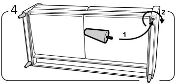
Mount them in place by twisting each clock-wise into the pre-drilled holes in each of the four.
