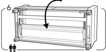
Mount the support legs in place by twisting each clock-wise into the pre-drilled holes.
