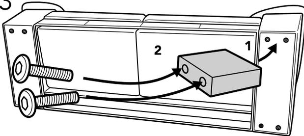
Mount the wood leg in place and screw the 2 (M6X25mm) bolts into the pre-drilled holes.
