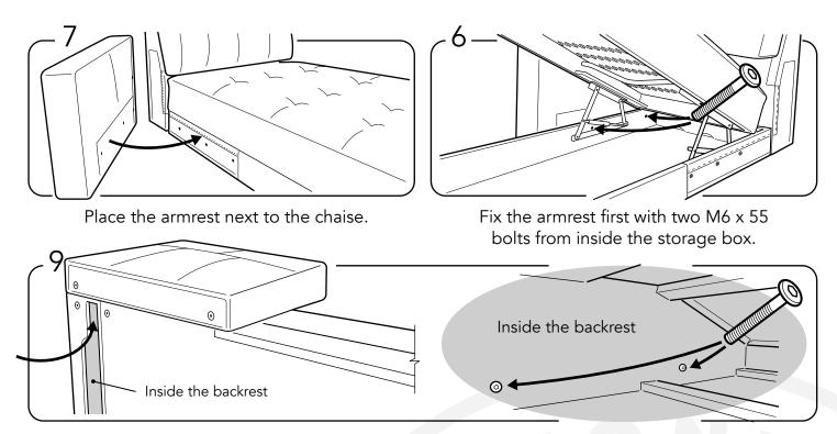
Close the chaise, turn it to the side and fix the armrest from inside the backrest with two M6  $\times$  55 bolts.
