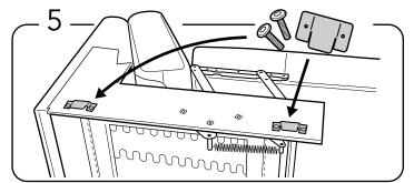
Attach previously unmounted metal brackets with M6  $\times$  20 bolts to the sleeper chaise side.
