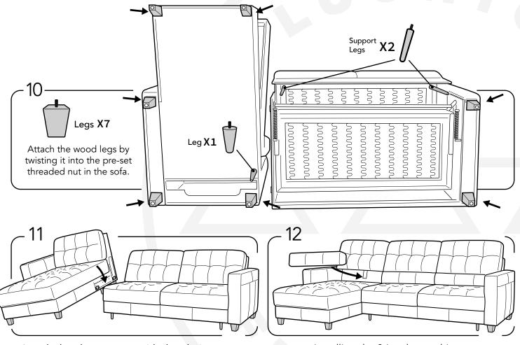
Attach the sleeper part with the chaise part as shown on picture. Be sure that the both metal brackets are attached correctly!
