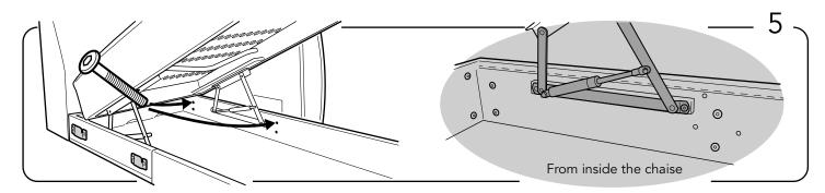
Fix the armrest first with four M6 x 55 bolts from inside the storage box.
