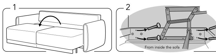
Open the mechanism completely.
