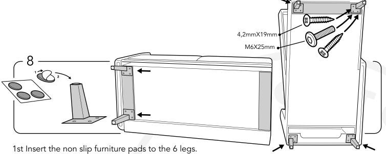
2nd Attach each legs with the M6x25mm bolt to align the metal in place then use two screws on each leg. 3rd Turn the sofa and chaise back to the legs.
