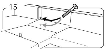
Put down the bed headside part and attach the bed backside to the corner part.
