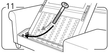
attach the 2 frontside armrest fixating bolts.
