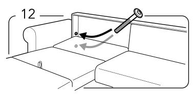
Put down the bed mechanism and attach the 2 backrest fixating bolts.
