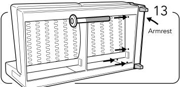
In the stationary part start with relocate the armrest in the opposite side and attach it with the 4 bolts as showen.
