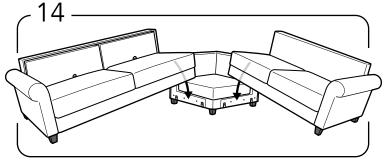
Attache the bed and the stationery parts to the corner part inside the pre-installed anchors.
