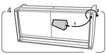
Mount them in place by twisting each clock-wise into the pre-drilled holes in each of the four.
