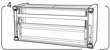
Mount the metal leg in place and screw the 4 (3,5mmX25mm) woodscrews.
