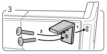
Mount the metal leg in place and screw the 2 (M6X25mm) bolts into the pre-drilled holes.
