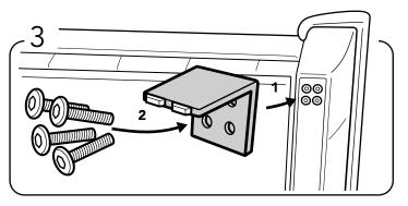
Mount the metal leg in place and screw the 2 (M6X25mm) bolts into the pre-drilled holes.
