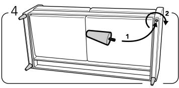
Mount them in place by twisting each clock-wise into the pre-drilled holes in each of the four.
